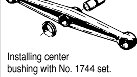
Installing center bushing with No. 1744 set.
